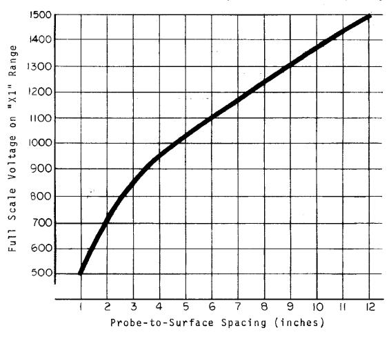
NOTE: Measured data taken using a 72" square metal surface.
